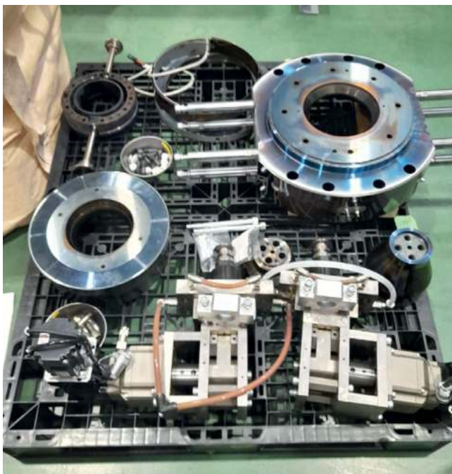
Picture 5: Components of the Asian copy of a PWDS-system that has been dismantled from the head (left side) and GWDS-die and GWDS-mandrel that have been attached to the head instead (right side)
