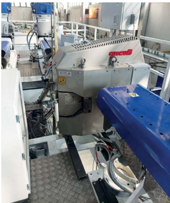
Production line with Gneuss RSFgenius filtration system in Europe
